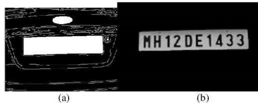
Fig.4.2.a.ii: (a) Filled image (b) Detected license plate
