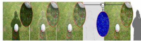
Fig. 8 Shadow Removal Steps (from left to right) (i) An original image with shadow. (ii) An initial estimate of the shadow-less image using a multi-level color transfer strategy. (iii) Improved estimate along the boundaries using in-painting. (iv, v and vi) The Bayesian formulation is optimized to solve for \alpha (iv) and \beta matte (v) and the final shadow-less image (v).
